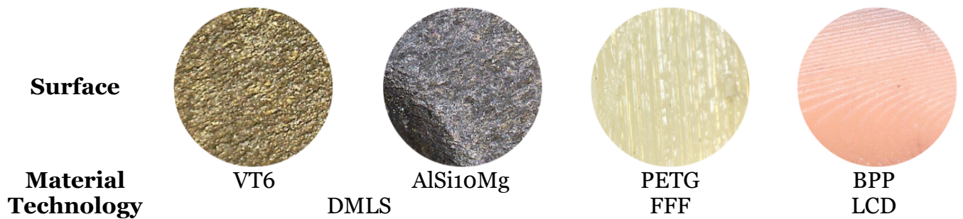
Fig. 10. Examples of surface topography of the tools' parts
